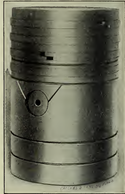
FIG. 2. PISTON, SHOWING OILWAYS
